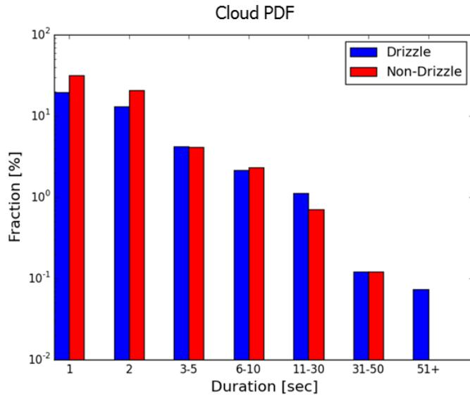
845 **Figure 5.** The probability density function (PDF) of drizzling and non-drizzling sections of liquid clouds from 20 flights observations of three consecutive winters (Jun - Oct, 2013 - 2015). The cloud distributions are analysed by consistent drizzle or non-drizzle cloud sections for each time period (e.g. 11-30 s).
