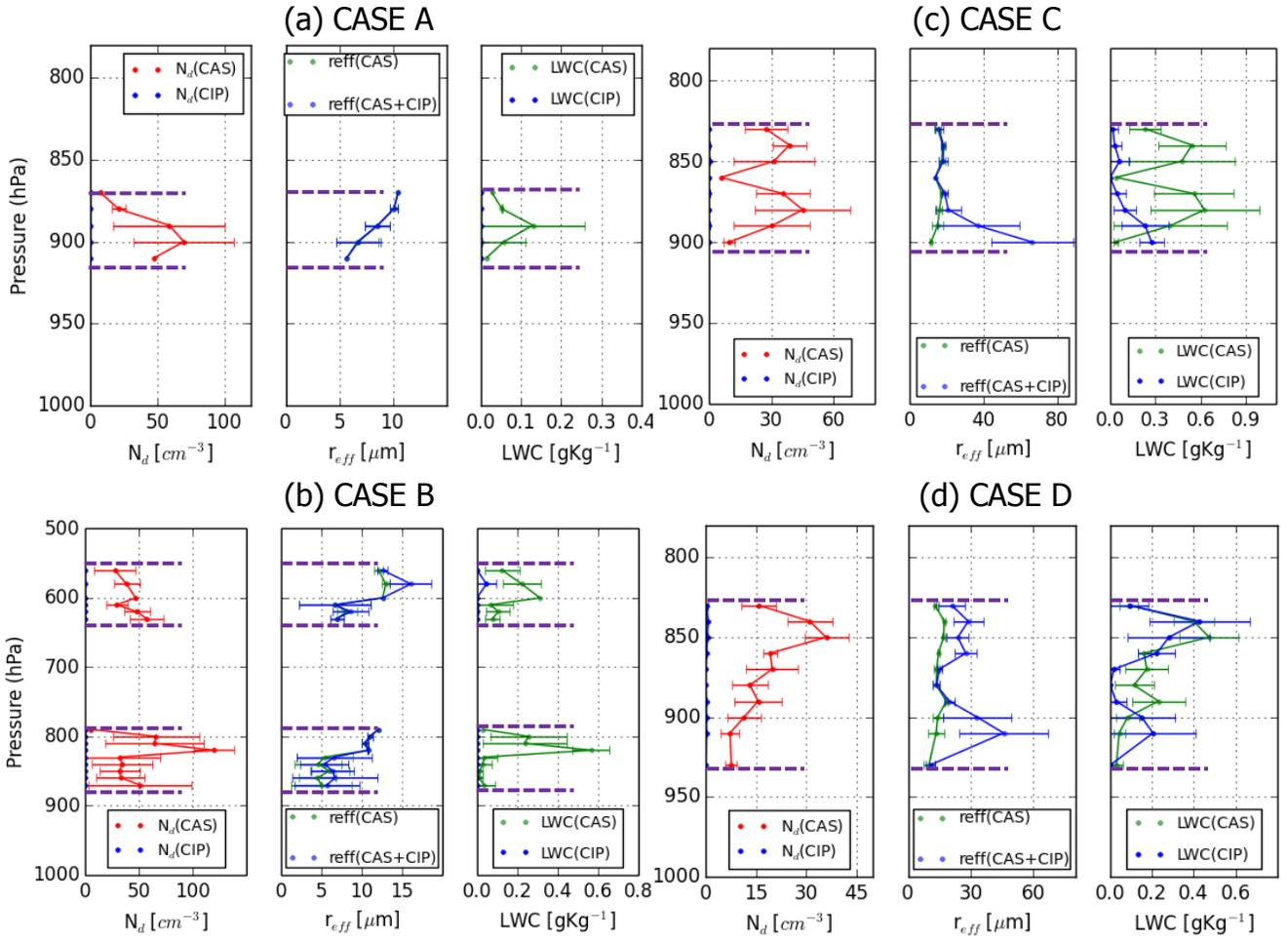
865 **Figure 8.** (a) – (d) Vertical profile of cloud microphysical properties ( $N_d$ ,  $r_{eff}$ , and LWC) from the soundings of non-drizzling cases (CASES A and B) and drizzling dominant (CASES C and D) flights in Figure 7(e) ~ (h). The estimated cloud base and top heights are indicated by the dashed lines. The error bars are standard deviations.
