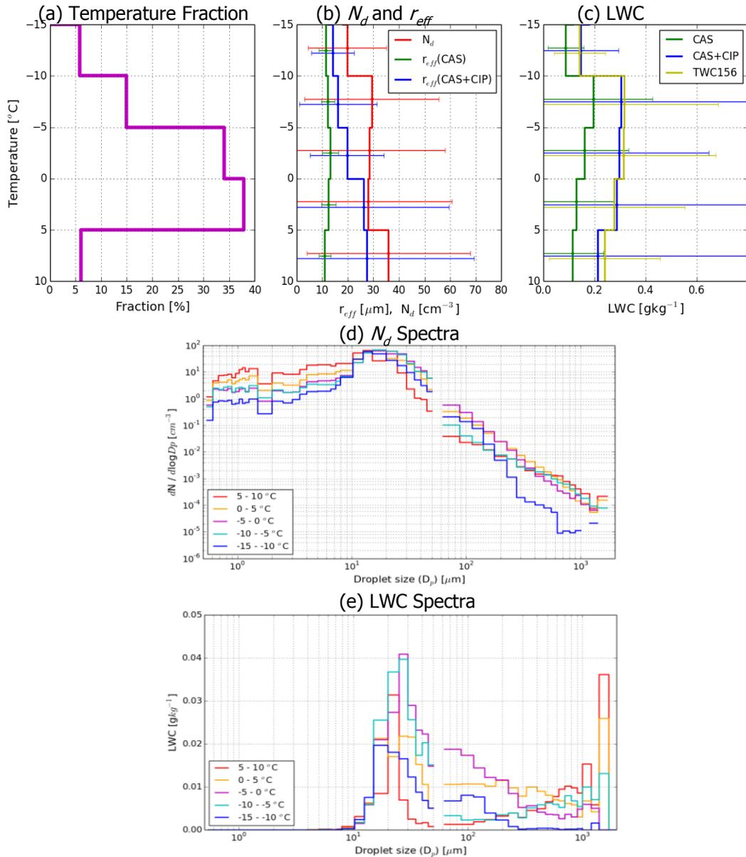
835 **Figure 3** Averaged microphysical properties and spectra by temperature for liquid clouds from
