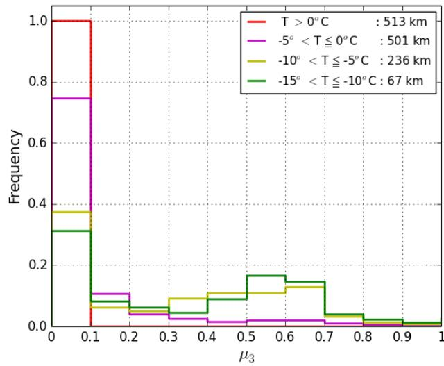
Figure 2. Fractions of cloud phase coefficient ( $\mu_3$ ) for different temperature intervals for 20 flights of three consecutive winters (Jun - Oct, 2013 - 2015).
