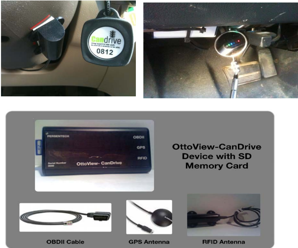
Figure 1. Multiple Views of ICRD (key chain fob in upper left; OBDII connector in upper right; actual device with memory card, OBDII cable, GPS antenna, and RFID antenna in lower portion of figure; from Porter et al., under review)
