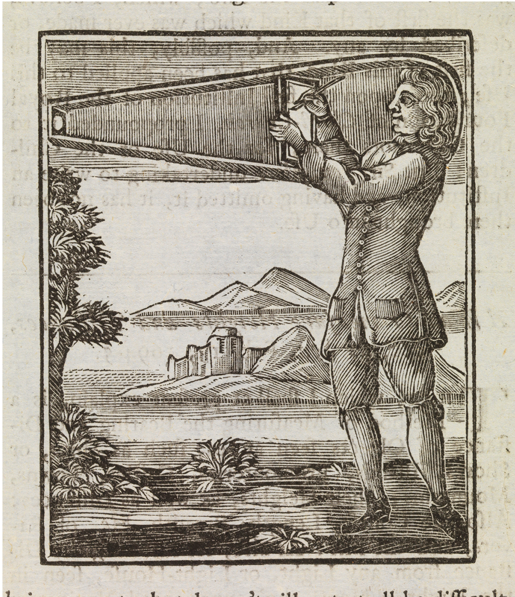
Figure 5. Robert Hooke's Drawing Instrument. "An Instrument of Use to take the Draught, or Picture of any Thing. Communicated by Dr. Hook (sic) to the Royal Society Dec. 19, 1694".
