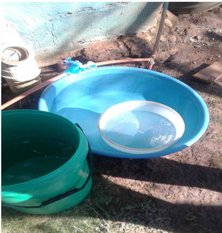
Figure 4.3a: The reported water leak with water being collected to estimate the amount of water that was being lost ( source author )
