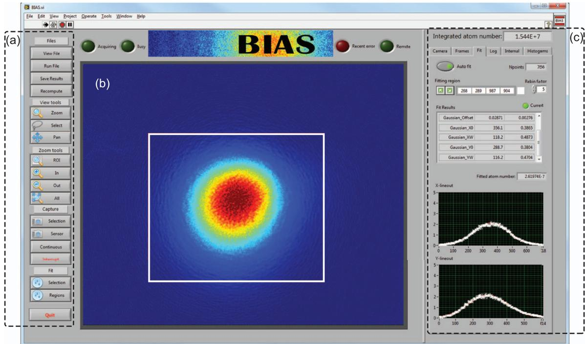
FIG. 6. The BIAS interface displaying a laser cooled atom cloud. (a) Manual controls for loading and capturing images, selecting regions of interest and zooming. (b) Computed optical depth (OD) image of the atoms, with a region of interest (white) selected for fitting. Multiple regions of interest may be selected for multi-component atom clouds. (c) Atom number and cloud size are displayed for immediate feedback.
