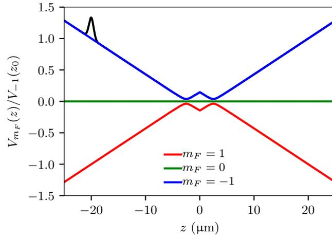
Figure 6.8: Adiabatic potentials for scenario II, with two closely spaced coupling regions. The initial probability distribution of the atoms is depicted (in arbitrary units), offset for clarity by the adiabatic potential of the initial state.
