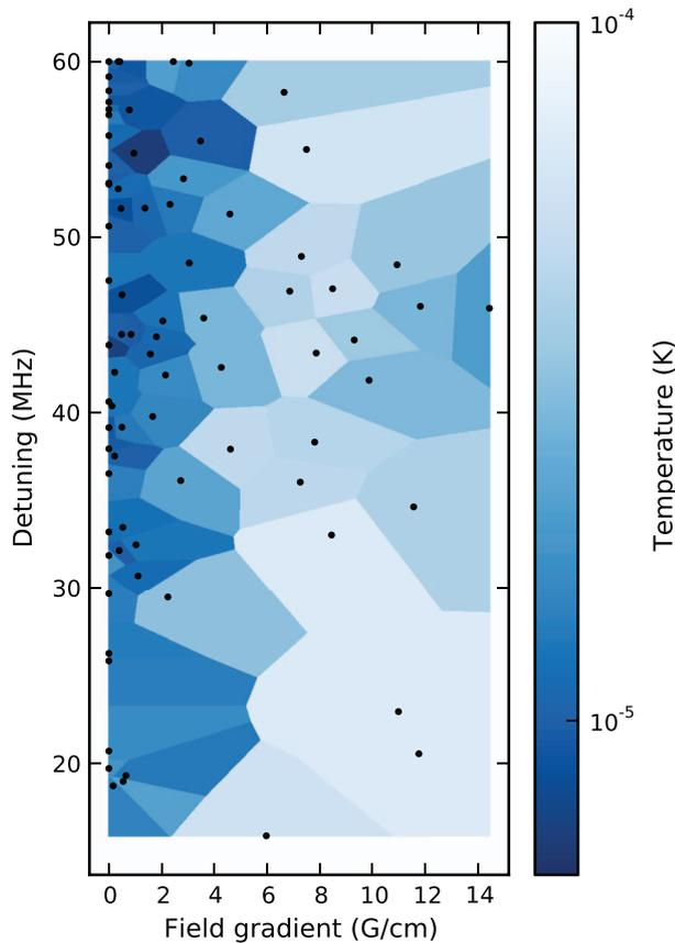
FIG. 9. A proof-of-principle optimization using *mise*. *mise* scanned the parameter space described in Sec. V, searching for the coldest point. Each black point represents a temperature measurement at a specific field gradient and detuning, with the surrounding shading indicating the temperature. Eighty points were taken, corresponding to 400 shots. The colder region of parameter space is sampled more densely than the uniformly-sampled scan, shown in Fig. 7(e), with 500 shots.
