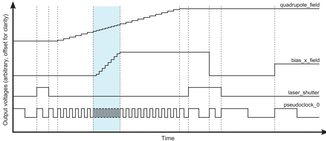
FIG. 2. An example of digital and analog voltage outputs generated by the `labscript` code in Fig. 3. The pseudoclock (lower trace) ticks when a digital output must change, or at the requested sample rate for time-varying analog outputs (upper two traces). Dashed vertical lines indicate a change in the pseudoclock frequency. When multiple analog outputs are varying at the same time (shaded region), the pseudoclock ticks at the highest of their sampling rates.
