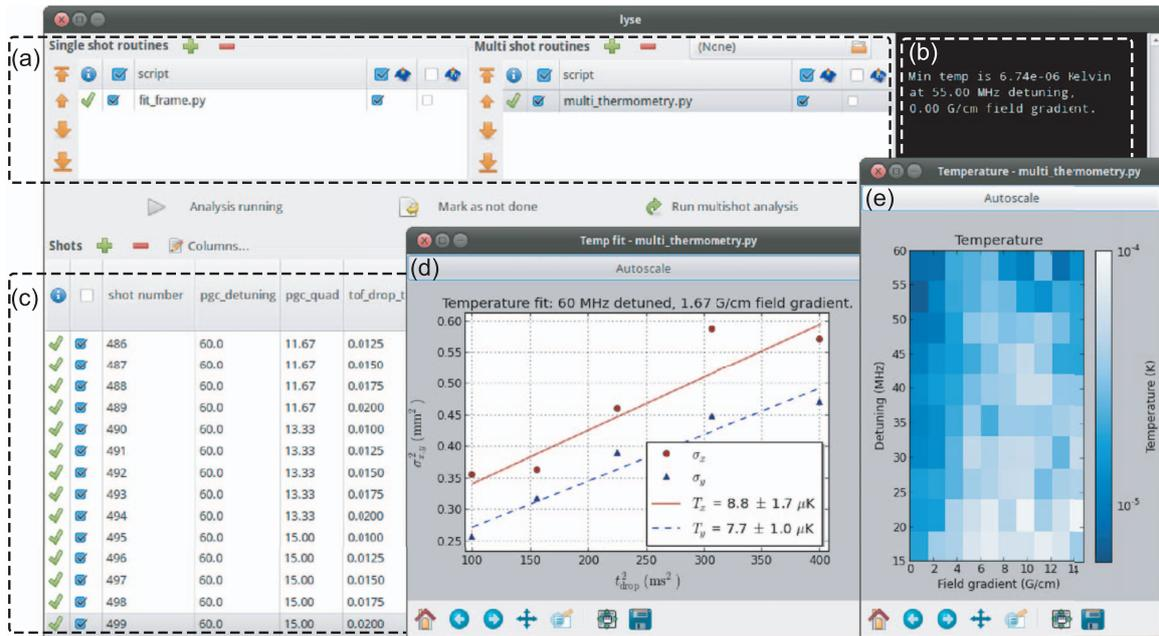
FIG. 7. The *lyse* interface. (a) Routines can be selected to analyze single or multiple shots. (b) Terminal output from the analysis routines in (a). (c) Table of shots; columns show globals and analysis results. A small subset of columns is displayed here. (d) A fit yielding the temperature of laser cooled atoms prepared at a particular field gradient and detuning. (e) The results of the analysis in (d) repeated at each point in the parameter space.
