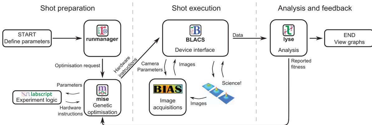
FIG. 8. The data flow for closed loop optimization. In contrast to Fig. 1, analysis results are used to determine future shots automatically. The optimizer *mise* varies parameters, directly calling *labscript* to compile new experiment shots. Parameters to be optimized are selected by the user in *runmanager*. *lyse* reports fitness to *mise* which is used to create the next generation of shots.
