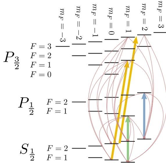
Figure 5.14: The full cooling scheme, including repump lasers (yellow), cooling lasers (blue and green), and all possible decay paths (red). The repump beam which is drawn in between two ground and excited states has a frequency equal to the average of those two transitions.
