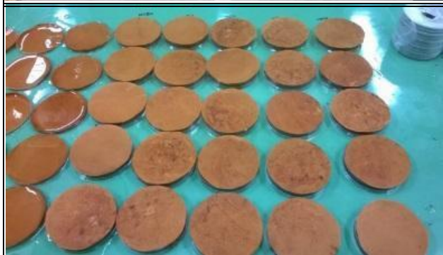
C) Deployment of phosphorus by a good contact of soil surface and wetted filter papers
