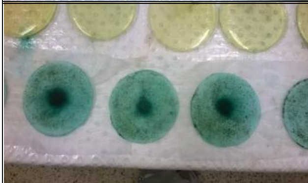
E) Staining the filter papers by soaking in Malachite green in HCl solution
