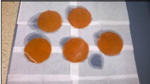
B) Impregnation of filter papers with iron oxide by soaking the filter papers in iron oxide solution at least for 15 minutes
