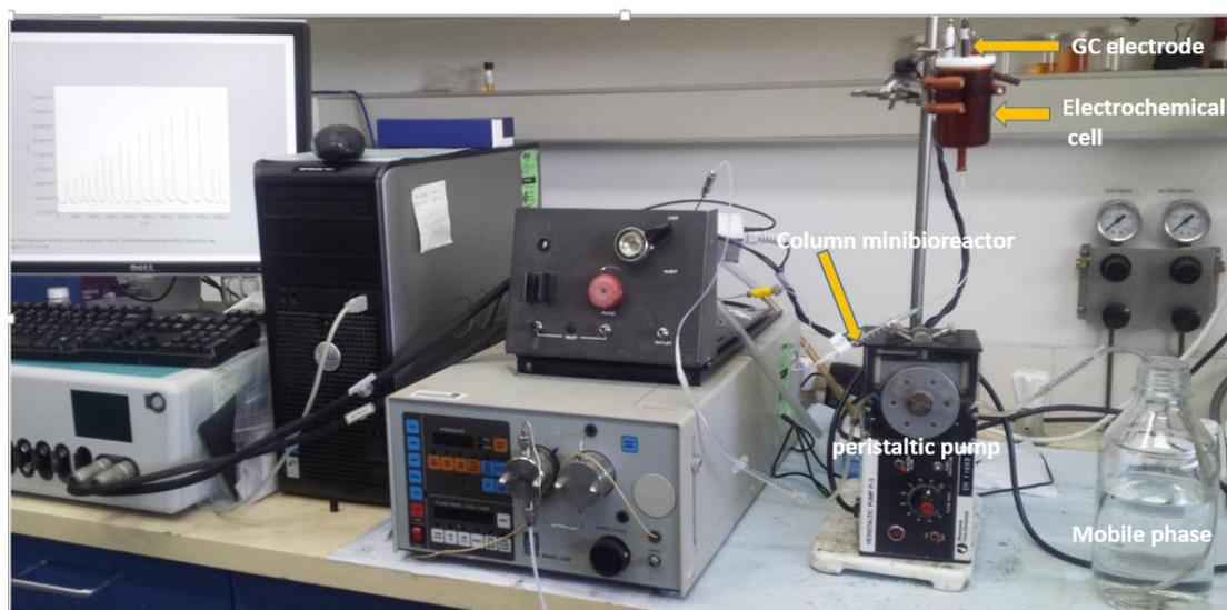
**Figure 4.22.** The FIA used for electrochemical measurements
