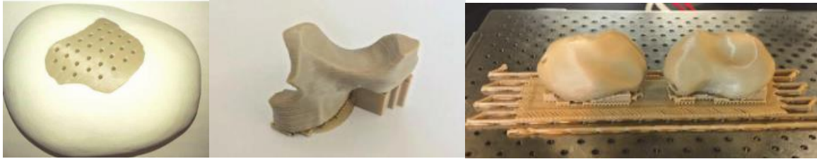
Figure 68. Patient specific implants printed in polyetheretherkone. Cranial defect (left), maxillary-zygomatic implant (centre) and scaphoid bone replacement (right) (Honigmann, Biomed Res Int, 2018)
