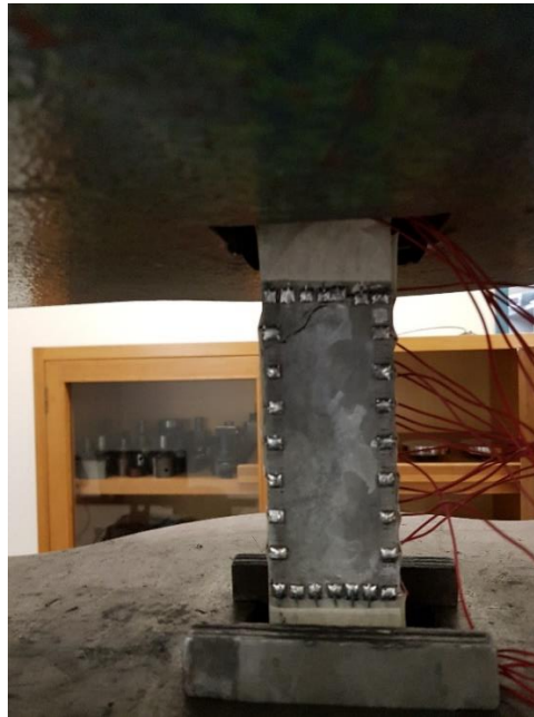
Figure 7.13 Crack pattern for crack exceeds monitoring area in tensile test.
