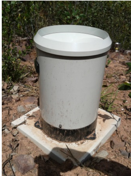
Plate 4-1. Pluviometer installed at study site. Photo was taken prior to installation of shade cloth border to attenuate splash erosion from adjacent bare soil surfaces. Note the evidence of rainsplash erosion and deposition on the outside walls of the instrument. Regrowing seedlings seen in the background of photo were trimmed regularly to prevent any interference with accurate rainfall measurement.
