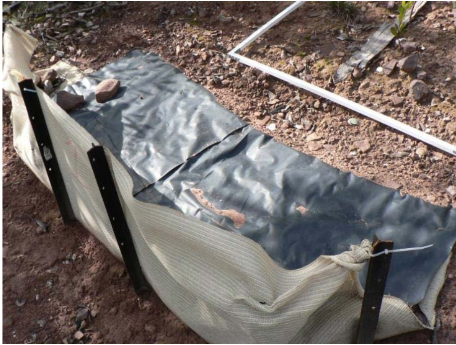
Plate 4-4. Sediment fence (#1) installed at the study site. Width of collecting area was 1.5 m. The large rocks seen on the left of the image were used to weigh-down the black impermeable sheet to maintain a relatively flat and smooth surface flush with the thin, rocky soil surface.
