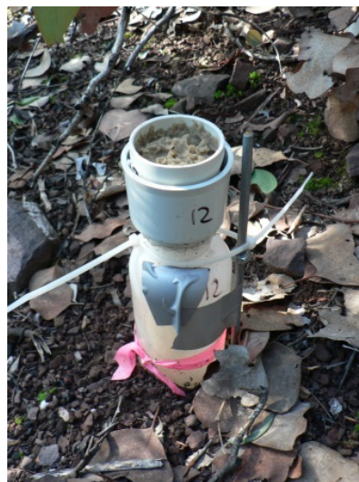
Plate 4-2. Splash cup assembly deployed in the field.
