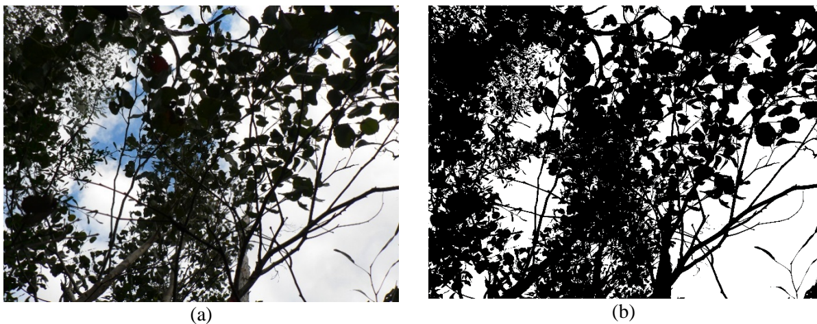
Figure 4-2. Sample image used to obtain canopy cover percentages: (a) Original photograph (note small patch of blue sky in background amidst generally overcast conditions); and then (b) Thresholded 8-bit binary black and white image processed in Image J software.
