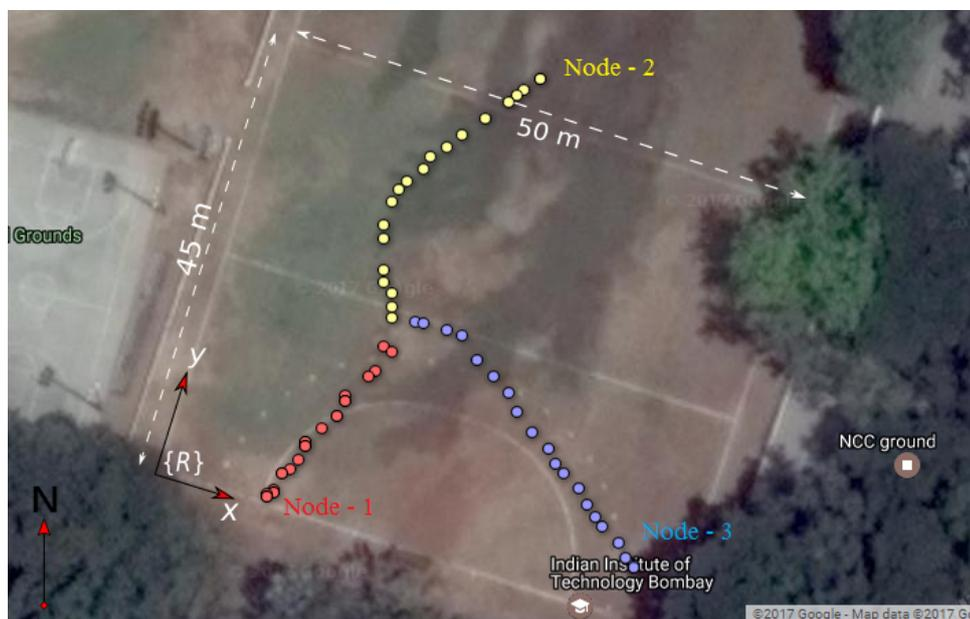
Figure 6.10: GPS plot of consensus between three physical quadrotors
