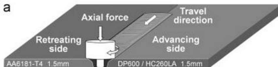
Figure. 2. 4 Schematic illustration of stir friction joining between Al alloy and high strength steel [84]
