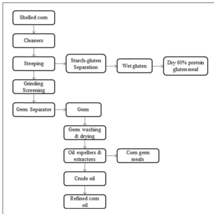
Fig. 2. Schematic diagram of corn oil extraction
