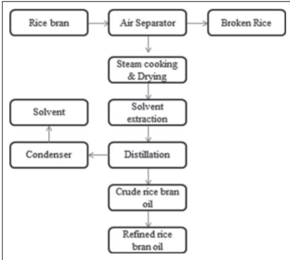
Fig. 1. Schematic diagram of rice bran oil extraction
