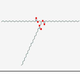
The diagram shows the chemical structure of Tribehnin. It consists of a central glycerol backbone (represented by a vertical zigzag line) esterified with three behenic acid chains (represented by horizontal zigzag lines). The ester linkages are highlighted with red boxes.   |
