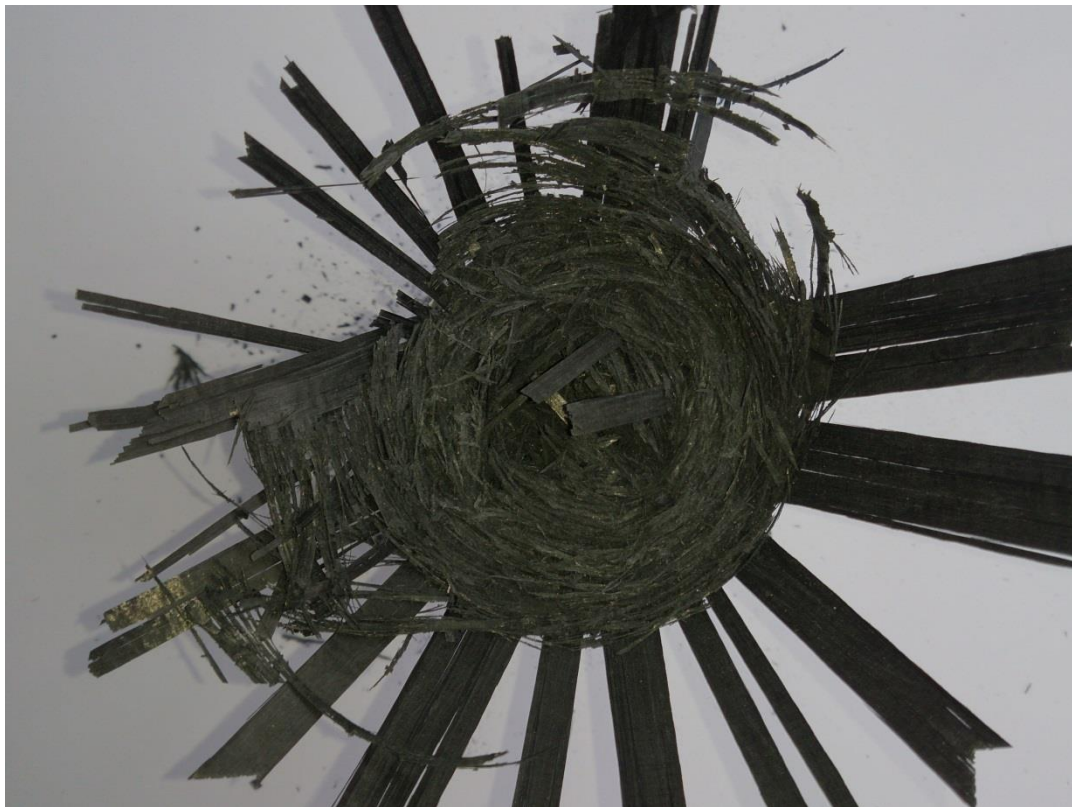
Figure 5.30: Post-test view of dynamic specimen showing concentration of debris near the centre.
