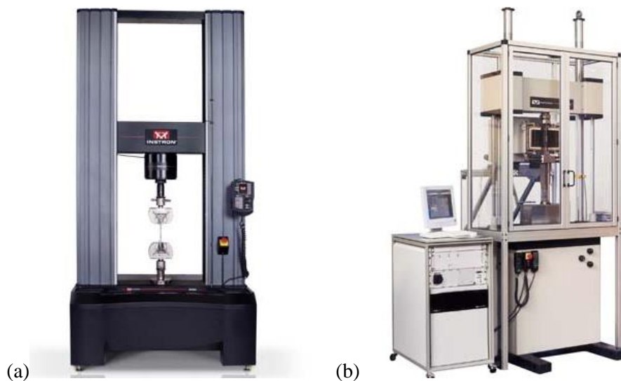
Figure 5.11: Screw-driven (a) and hydraulic testing machine (b) used in this study.
