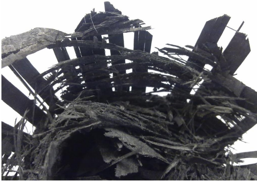
Figure 5.19: Close-up of fragmentation of the internal plies.
