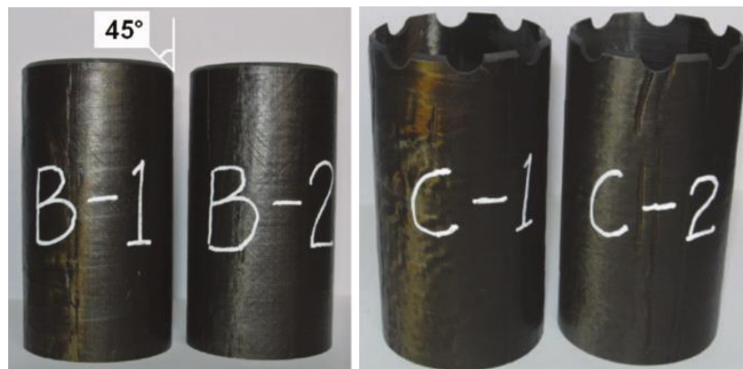
Figure 5.2: Specimens showing manufacturing defects: creases along a seam (B-1) and wrinkling of the ply (C-1 and C-2).
