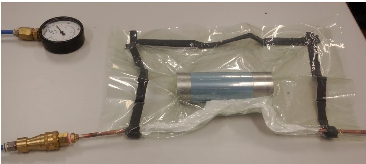
Figure 5.5: Debulking in vacuum bag after applying low heat.
