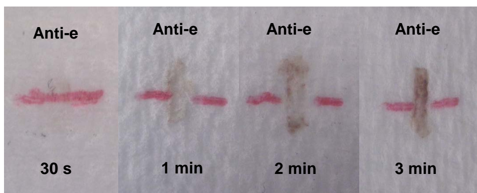
Figure 3. Increasing degrees of haemagglutination of the second group e in antibody-treated paper as a function of time.
