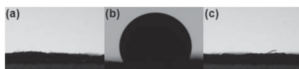
Figure 7. Profile of blood in/on (a) paper; (b) antibody paper (contact angle = 122.2°); and (c) plasma treated antibody paper. (a) Kleenex paper square without any treatment. (b) Kleenex paper square treated by adding antibody solution twice. (c) Kleenex paper square treated using the same treatment procedure as blood typing paper. Four microliters of blood was deposited onto each paper square respectively. After 3 s, images were taken to compare the status of blood sample on each paper. Blood penetrated into paper (a) and plasma treated antibody paper (c) in less than 3 s. However, water does not completely penetrate into antibody paper (b) within 30 s.
