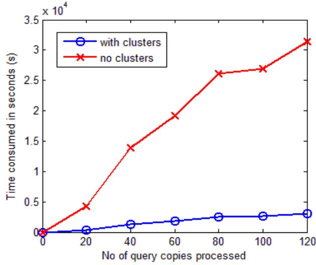
**Figure 5.8.** Time consumed corresponding to the number of query copies processed by using scalable color
