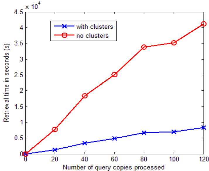
**Figure 5.6.Time consumed corresponding to the number of query copies processedby using edge histogram**
