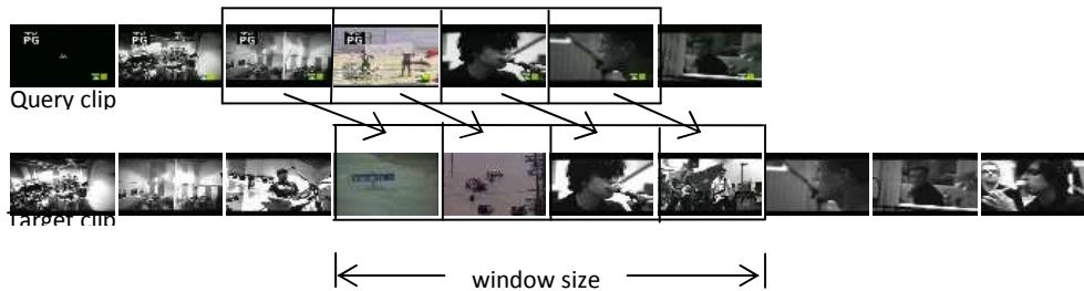
**Figure 4.6.Overview of the sliding window-based similarity technique**
