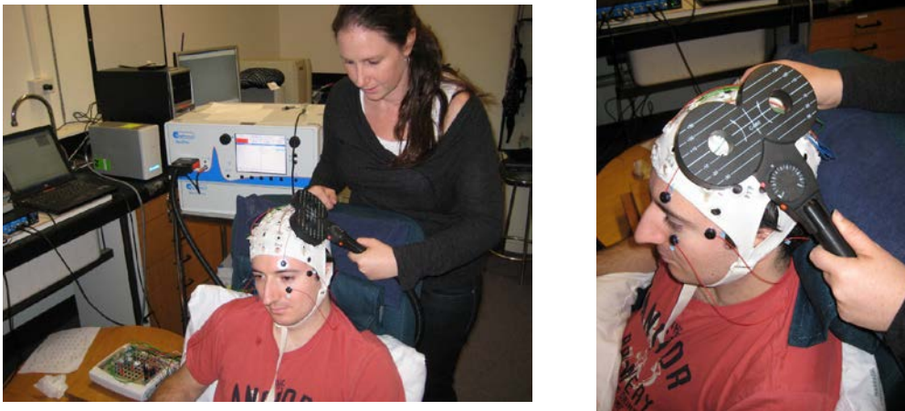
Figure 1. The combined Transcranial Magnetic Stimulation-electroencephalography (TMS-EEG) technique set up. The TMS-EEG set up of the current study; including the figure-8 coil, the EEG system and the MagVenture brain stimulation power source. Images supplied by Monash Alfred Psychiatry Research Centre.
