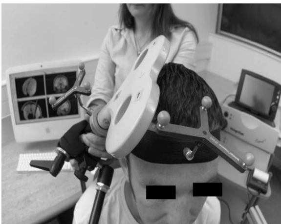
Fig. 1. Transcranial magnetic stimulation (TMS) application using a figure-8 coil over the motor cortex. The TMS figure-8 coil is placed over the subject's right motor cortex using a mechanical coil holder. A brief electric current passes through the magnetic coil which induces a transient magnetic pulse. This pulse penetrates through to the underlying cortex and generates an electric field within the targeted cortical regions which can induce depolarization of superficial cortical neurons and in this case activate muscles of the left hand if the intensity used will be above the motor threshold. Repetitive TMS can result in stimulation and disruption of local neural activity in the region beneath the coil and interconnected areas. Images courtesy of The Magstim Company Limited.
