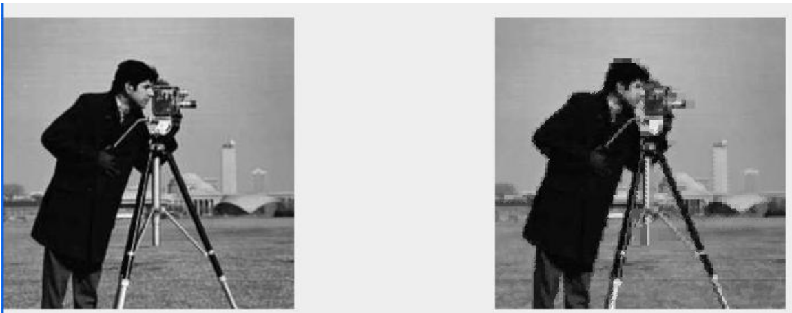
Figure 9. Wedgelet representation (right). The smallest wedgelet is 2^3 \times 2^3 .
