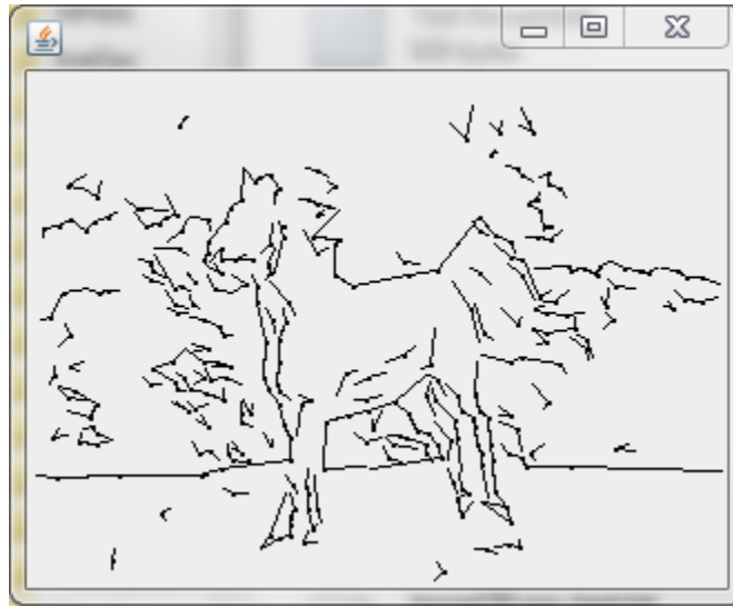
Figure 41. Image shows the extracted turning points and the straight edge linking them. These are the features used for detecting the target object in recognition.
