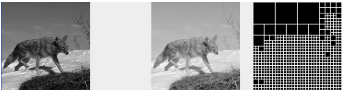
Figure 16. Original image (left). Combined wedgelet and Tchebichef decomposition and reconstruction (middle). The quadtree partitioning grid (right).
