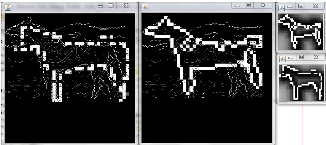
Figure 56. (Left) Path of the exemplar superimposed on the test image. (Middle) The constructed ant path over the wedgelet image. (Right) Paths superimposed on the distance transform of the exemplar.
