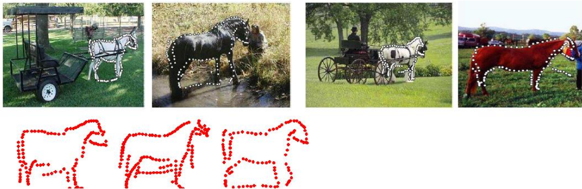
Figure 62. Contour detection using Pairs of Adjacent Segments (Ferrari et al 2010). (Top) Results of detection. (Bottom) Models used for detection.
