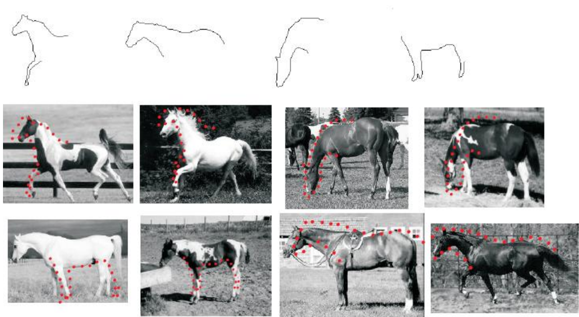
Figure 61. Contour fragment detection. (Top) Contour parts used for detection. (Bottom) Detection results using the Shape Band method (Bai, Li et al. 2009).
