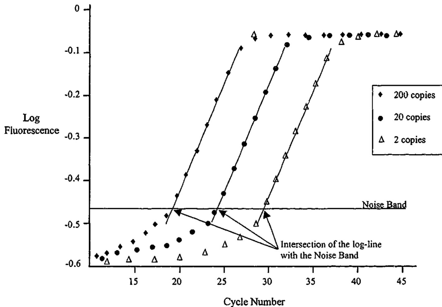
**Figure 4-2:** Quantification with the LightCycler. The graph shows the amplification of a target molecule at different concentrations, and the various points represent individual data points. The log-lines are extrapolated to the noise band line which defines the beginning of the log-linear phase. Significant differences in fluorescence can be seen in the log-linear phase of the PCR, whereas the fluorescence signal cannot be distinguished in the plateau phase.
