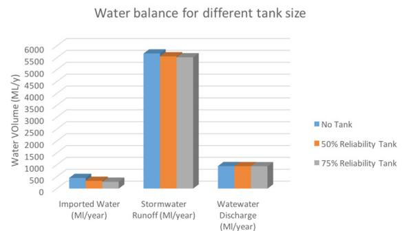
Fig. 8: Water balance for different tank sizes in Cibinong situ front city Aquacycle model
