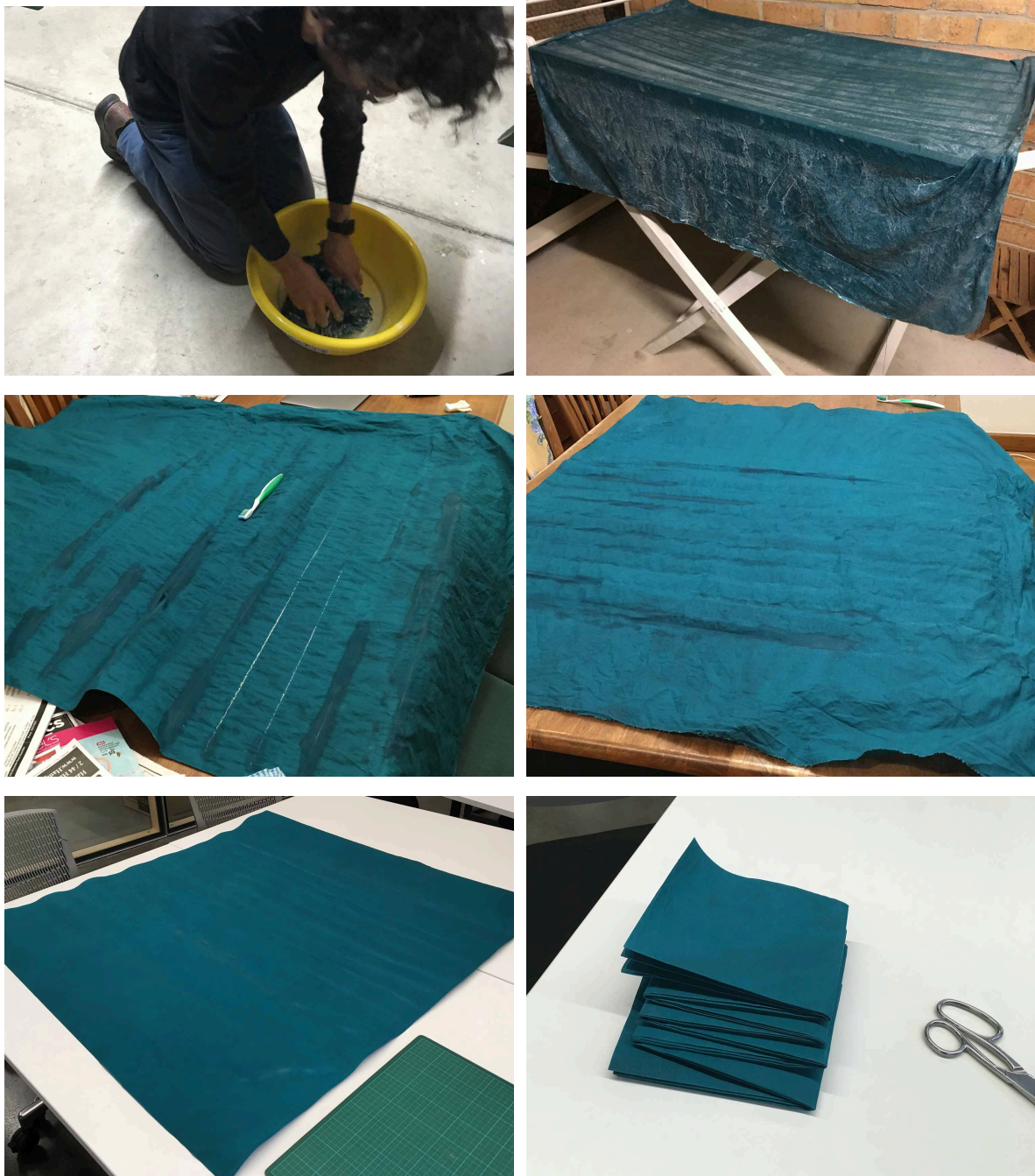
Figure C.9 Stiffening cotton broadcloth for folding, from left to right: soaking in 1:1 PVA glue and water solution; air drying; cleaning glue residue; cleaned sheet; ironed sheet; and Miura folded sheet for Computational Costume v2 [§ 4.3.5] (p.95) .
