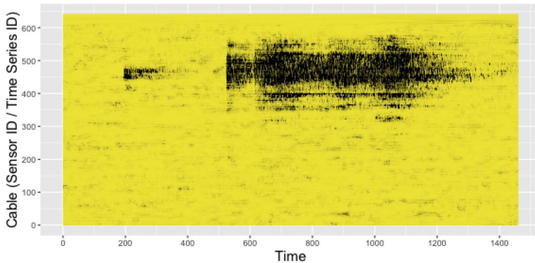
**Figure 1.** Multivariate time series plot of a dataset obtained using a fiber optic cable. Axis “Cable” represents individual points of the sensor cable. There are 640 time series each with 1459 time points. Yellow corresponds to low values and black to high values. The black region near the upper endpoint of the cable (around 350–500) indicates the presence of an anomalous event (e.g., intrusion attack, gas pipeline leak, etc.) that has taken place during the 500–1300 time period.
