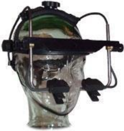
Figure 4. Eyelink II dark pupil, video-oculography system
