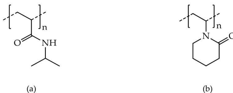
Figure 2.4. Chemical structure of (a) PNIPAAm; (b) PVCL.
