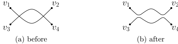
Fig. 4.12 Removing two crossings on two edges that cross each other an even number of times using the strengthened version of R_I^p .
