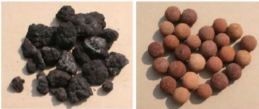
Figure 2-8 Different shapes of particles, left side is non-spherical particles and right side is spherical particles (Yoon et al., 2000)
