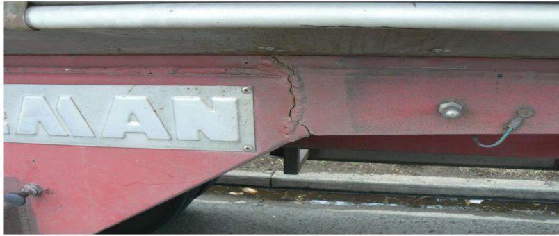
(b) Cracking at a welded joint in a bitumen tanker.
