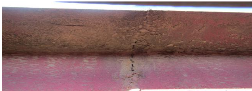
(a) A welded and re-cracked cracking in a log trailer frame.
