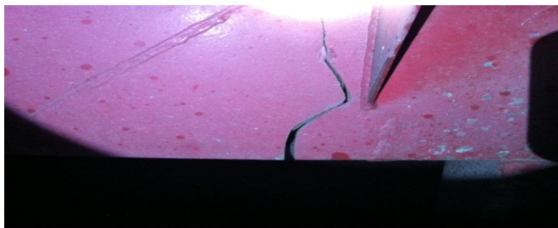
(a) Cracking at a tri axle trailer chassis.
