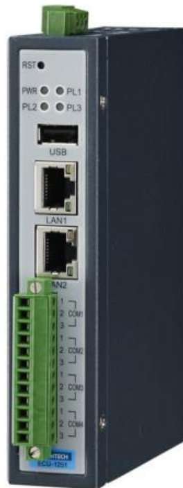
Figure 58 Advantech ECU1251 gateway for bridging the physical and cyber systems.
