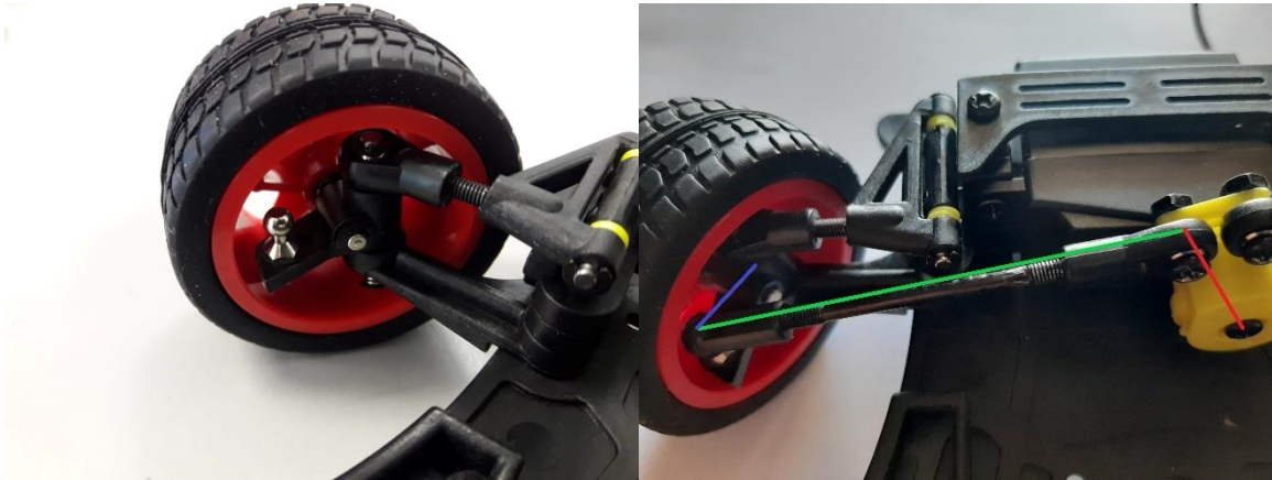
Figure 19 Left wheel with steering system showing the links of the steering system. The colors red, green, and blue correspond to link 1, 2, and 3 of the steering system for simulation.
