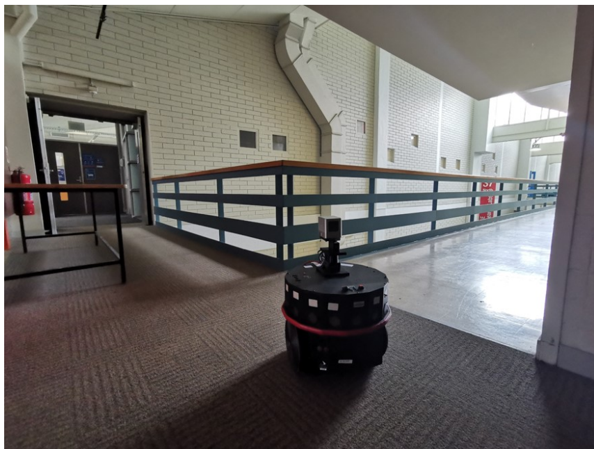
Figure 5.14 Designed challenges in the experiment: sharp turns with closing obstacles.
