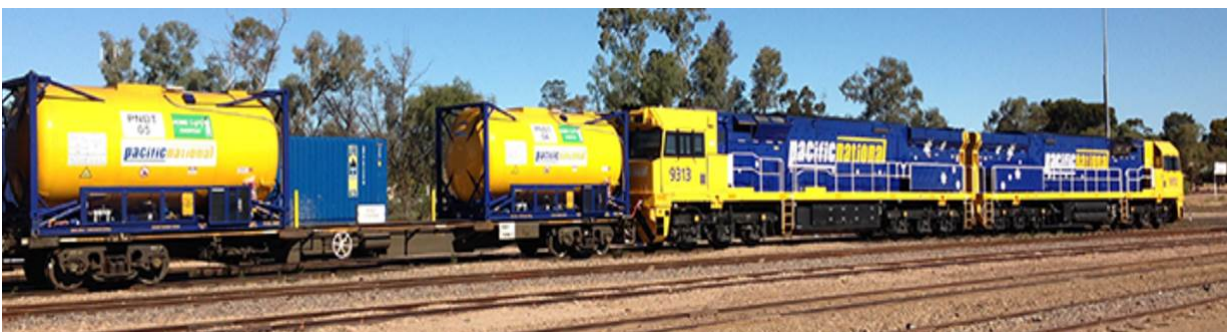
Figure 1.1: An example of inline refueling tanks. The picture courtesy of Pacific National Pty. Ltd., 2018.
