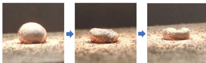
Figure 34 The removal of liquid from the Janus liquid marble via the substrate's hole tends to disrupt the uniform separation of the graphite and copper particles at the outset. The final outcome, however, is a structure that strongly deviates from a sphere.
