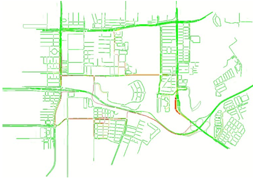
Figure 6.3. A snapshot of the SUMO simulation for Bandar Sunway
