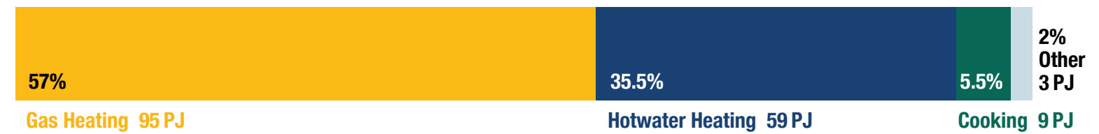
Figure 3: Residential gas consumption by end use
