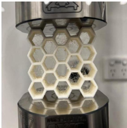
Figure 19 Setup of unidirectional compression test for a fabricated honeycomb sample.
