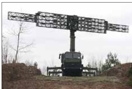
KBR Vostok E., fully deployed, showing the innovative Kharchenko loop antenna design.
