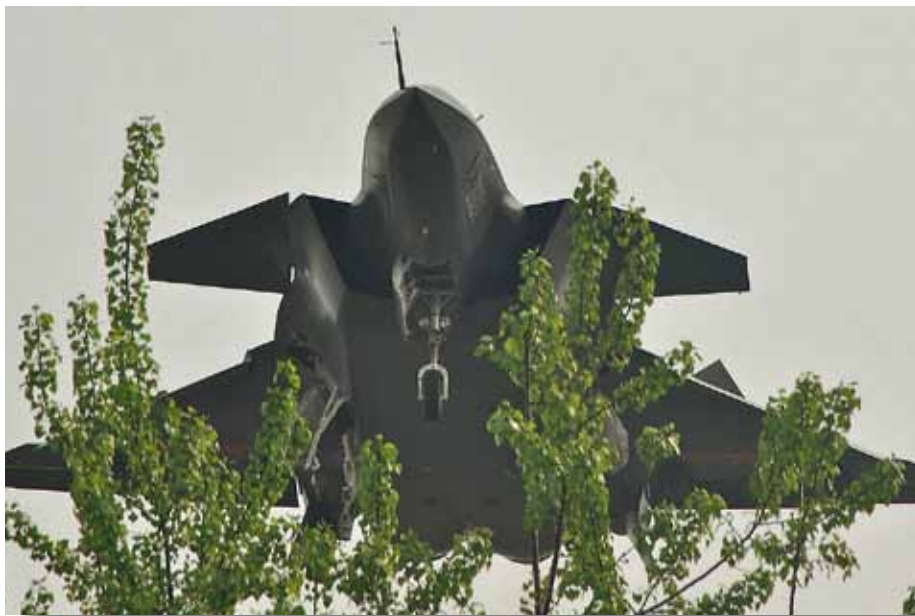
Detail of J-20 nose and inlet. The main weapon bay doors are discernable.
