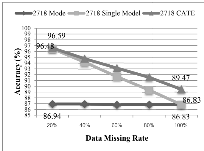
Figure 5-30: Accuracy of the single model and CATE framework approaches at specific missing data rates for road links 1206, 2613 and 2718
