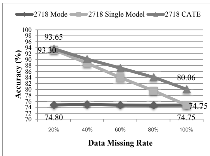
Figure 5-31: Accuracy of the mode, single model, and CATE framework approaches at specific missing data rates for road segments 1206, 2613 and 2718 (active period)
