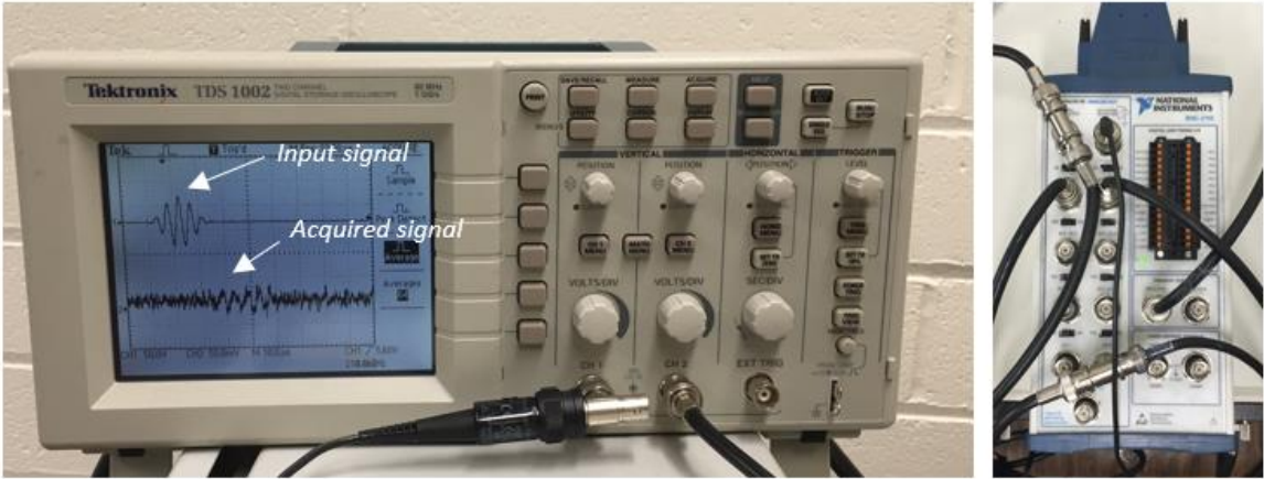
Figure 2.12: (LEFT) Oscilloscope showing input signal to the PZT and acquired signal via laser sensor (RIGHT) National Instrument BNC 2110 block
