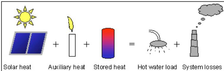
**Figure 5** An energy balance for a solar water heater
