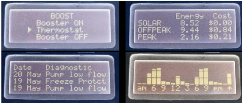
**Figure 7** Four images of display options from the local controller
